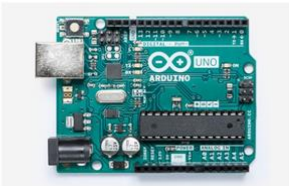
Fig1. Arduino Uno Rev3,Code: A000066
