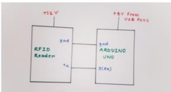
Fig 2. Interfacing Arduino with RFID
