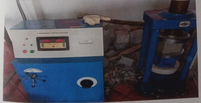
TESTING OF COMPRESSIVE STRENGTH OF CONCRETE
