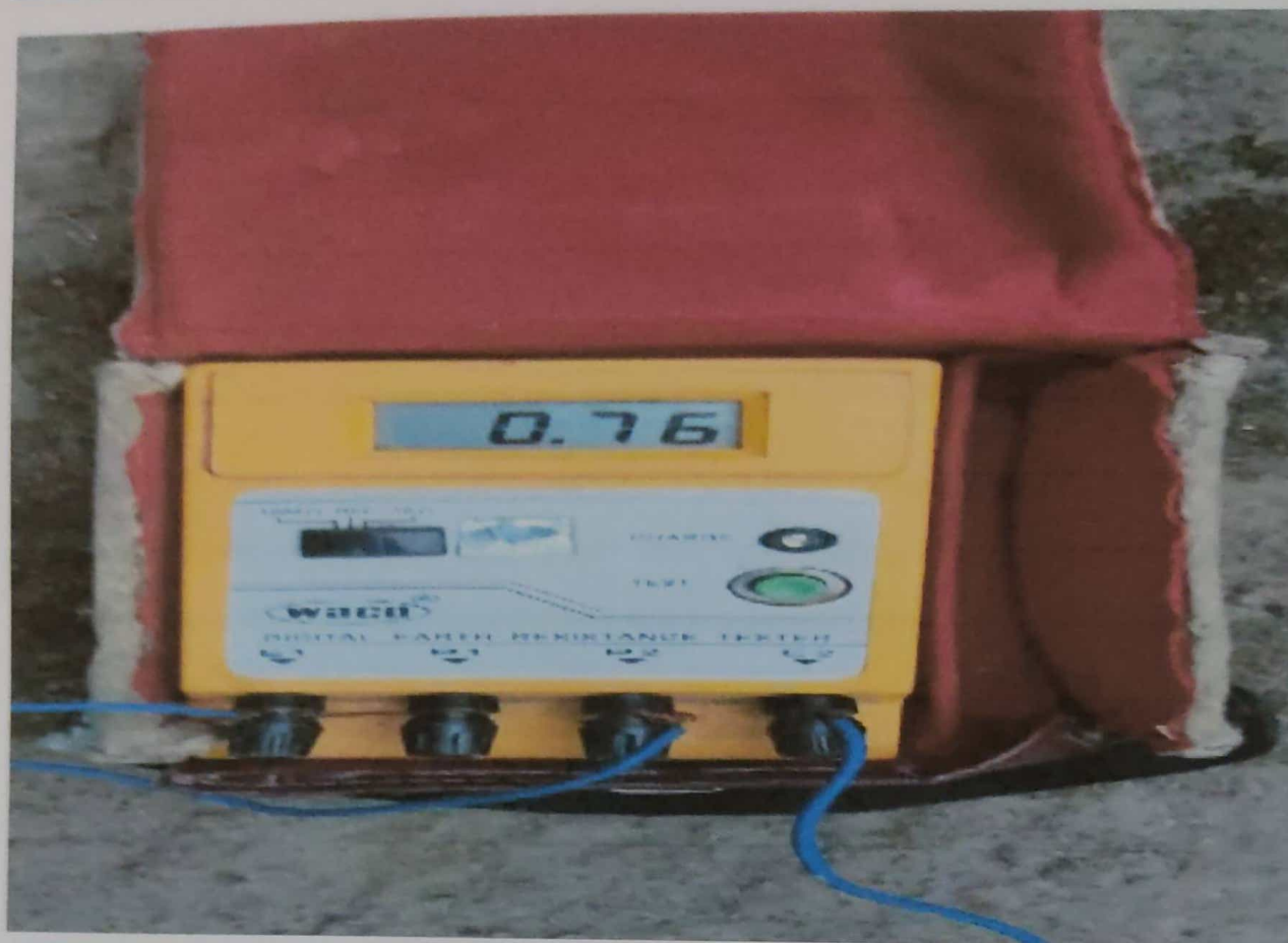
Fig 6 Earthing Pit Testing
